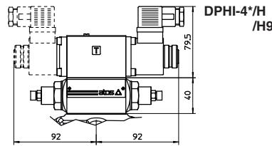
Overall dimensions refer to valves with connectors type SP-666
