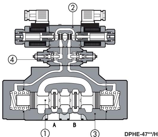
DPHI, DPHE and DPHER are spool ① type, two or three position, two stage directional solenoid valves.
