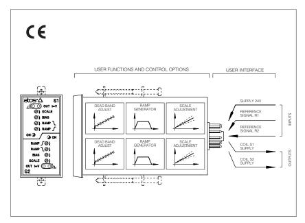
1 MODEL CODE AC – 01F E-BM E-BM = electronic driver Fast plug-in format set code (see 4.4) Series number AC = for prortional valves without transducer = 24 V<sub>DC</sub> power supply = 12 V<sub>DC</sub> power supply (see 4.1) 01F = for single solenoid proportional valves 011F = for two single solenoid proportional valves = standard symmetrical ramp 05F = for double solenoid proportional valves /RR = with adjustable dissymmetrical ramps
