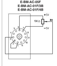
The internal ramp generator circuit converts a step input signal into a slowly increasing output signal (solenoid current). The rise/fall time of the current is set via potentiometers on front panel up to a max. time of 10 sec. for 0-100% of reference signal.
