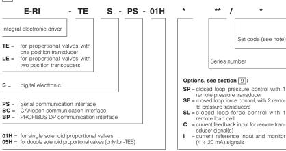
Note: the set code identifies the correspondence between the digital integral driver and the relevant valve; it is assigned by Atos when the driver is ordered as a spare part.
